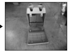
**STEP 4:** Remove (unsnap) the rear panel of the console.
